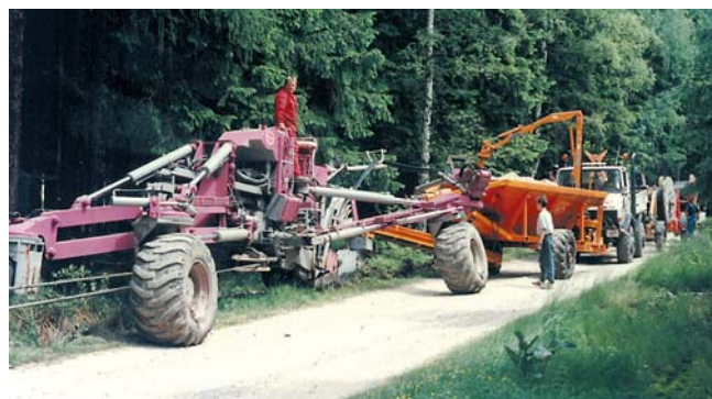
Laying a high-tension power cable by using the Automatic Sanding Cart
